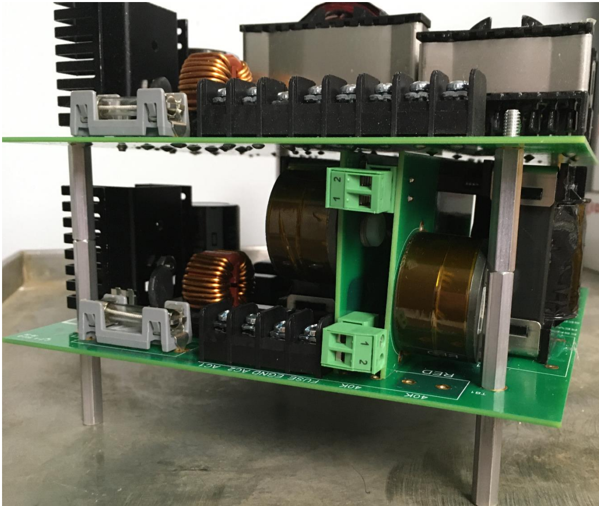
Figure 1: Improved Driver Board (bottom) in standard stacked configuration with older style driver board (top).
