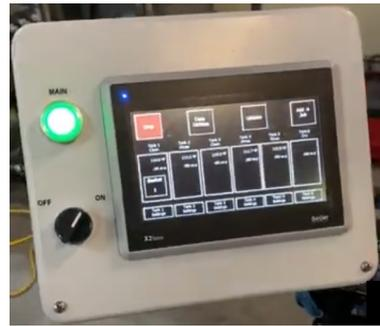
PLC-HMI for recipe creation and control of the ASTM967 passivation process.
