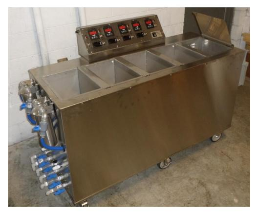
Multi-tank ultrasonic passivation system for: clean/rinse/passivate/rinse/(dry) applications
