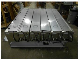
Multi-tank ultrasonic system for: clean/rinse/passivate/rinse/dry applications
