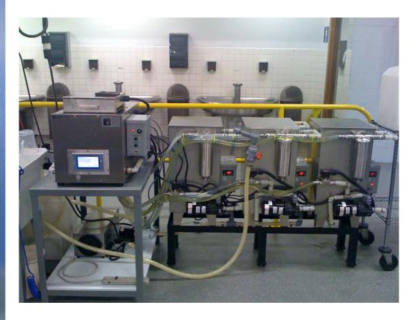
Completely closed, modular system incorporating integrated heated storage containment tanks with a self-contained, automatic ultrasonic washer
