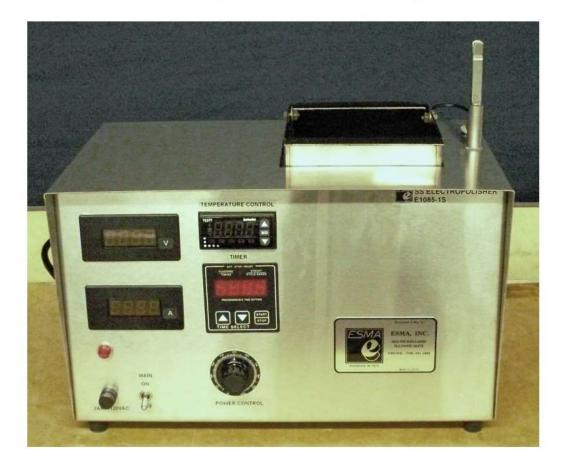
Benchtop electropolisher, all-in one system with variable voltage (DC) control and digital timer and temperature controller.
