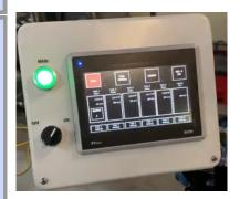
PLC-HMI for recipe creation and control of the ASTM967 passivation process.
