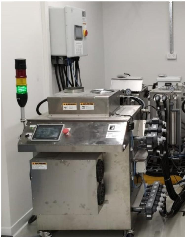
**Completely closed, modular system incorporating integrated heated storage containment tanks with a self-contained, automatic ultrasonic washer**
