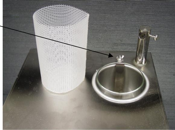
The polypro mesh liner is inserted **over** the cathode to eliminate the possibility of shorting the anode to the strip cathode.
