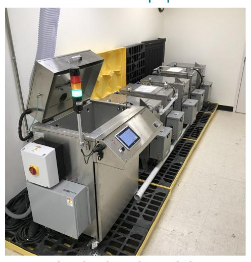
Completely closed, modular system incorporating integrated heated storage containment tanks with a self -contained, automatic ultrasonic washer
