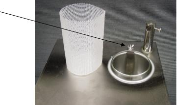
The polypro mesh liner is inserted **<u>over</u>** the cathode to eliminate the possibility of shorting the anode to the strip cathode.
